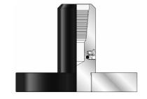
An integral bleed-off port is incorporated to allow for the possibility of bleeding down trapped residual CT pressure.
