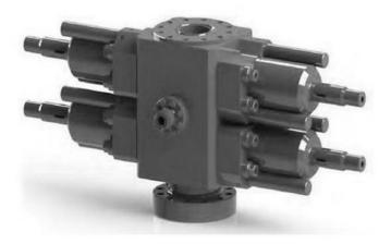
The Ram Assembled in the Combi BOP from upper to lower normally is Shear-blind Ram, Slip-pipe Ram. The Shear-blind Ram combines the function of Blind Ram and Shear Ram of the Quad Ram BOP. The Slip-pipe Ram combines the function of Slip Ram and Pipe Ram of the Quad Ram BOP. Other parameters of the Combi BOP is similar to Quad Ram BOP.
