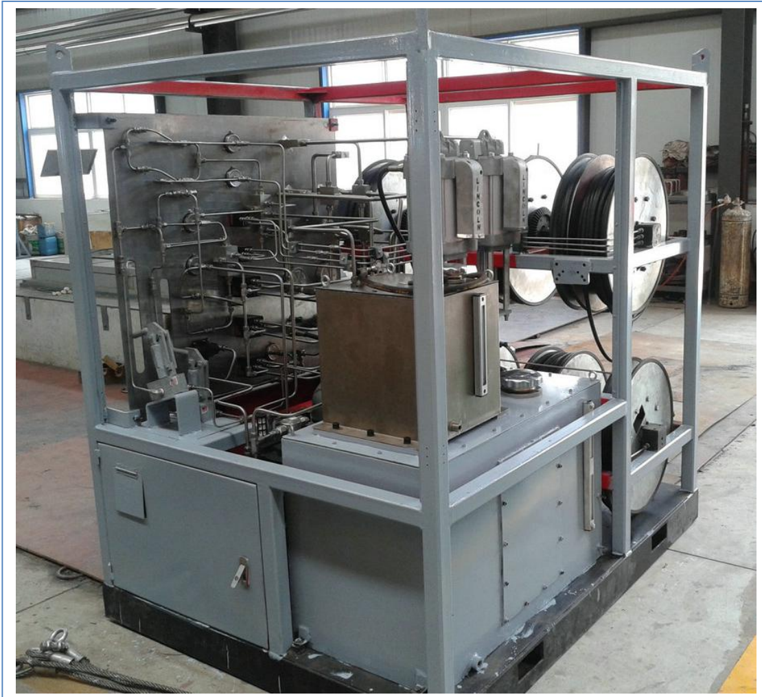
Grease and Hydraulic Control Module for Wireline PCE
